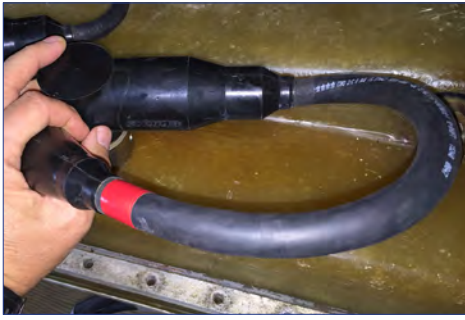
(Left) Rebuilt BIRNS 24-VDC cable assembly with 90° penetrator installed. (Right) Pisces IV exercising its robotic manipulators during a 1,500-m test dive off the coast of South Oahu October 2014.
